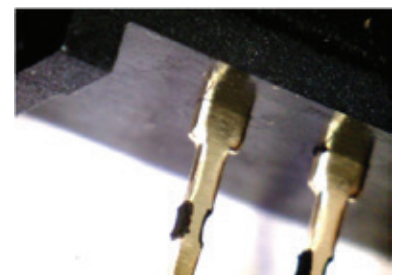
Black copper oxidation on contact leads.
