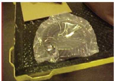
Zerust cold-seal film protecting a large gear for service shipment. Previously parts had been wrapped in VCI film and tape.
