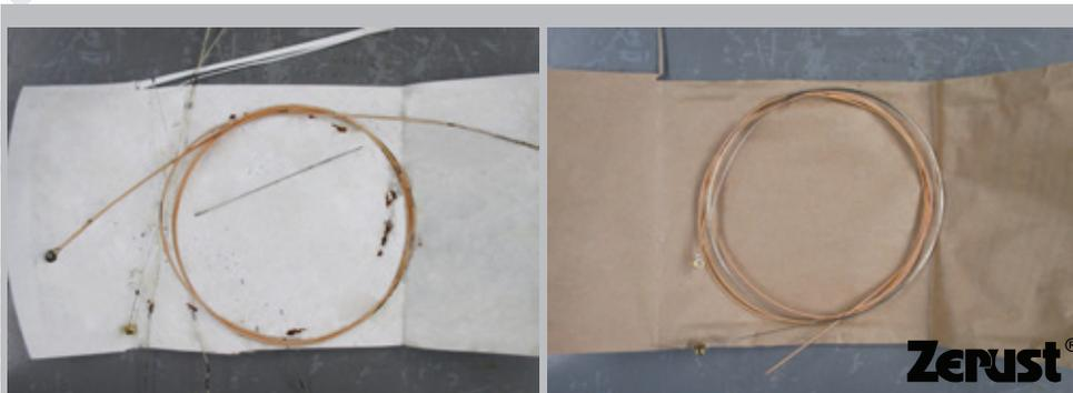
14 days in humidity chamber side by side test results. On left, existing VCI supplier, on right, Zerust VCI Envelope.
