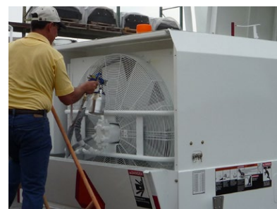
Zerust Axxanol Spray-G was applied for additional protection as an extra precaution in case of accidental rips or holes in the VCI shrink film over time.
