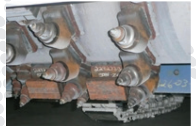
Non-critical area left unprotected by Axxanol Spray-G during shipment. Unprotected area quickly rusted.
