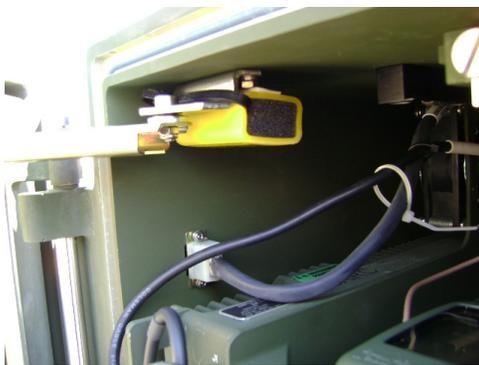
ZERUST® Vapor Capsules are a highly effective and economical solution for protecting military equipment and electronics. The mechanism involves the release of a corrosion-inhibiting vapor that forms a thin, invisible layer on the metal surface. This process, in turn, prevents rust and corrosion. Notably, this method is greatly beneficial to the military, ensuring both the integrity and longevity of their assets. As a result, this ZERUST® VCI technology is approved and trusted by the government.
