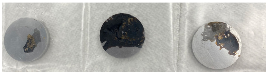
Figure 3 - As packaged and tested in plain polyethylene bags, Corrosion developed within 21 days of humidity exposure.
