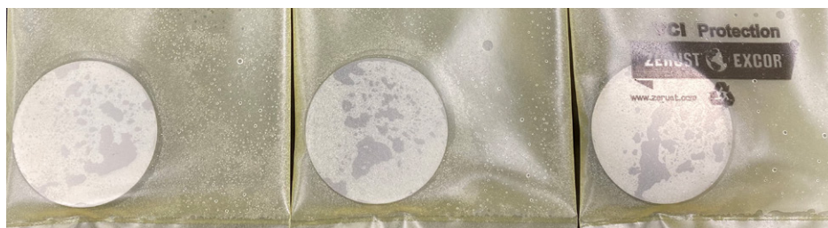
Figure 2 - As packaged and tested in Zerust® ICT®510-C Ferrous bags, 90-day humidity exposure result; No Visible Corrosion
