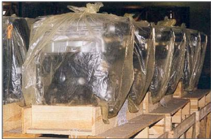
Figure 2 – Engines in sealed VCI bags during long-term storage and subsequent ocean shipment.
