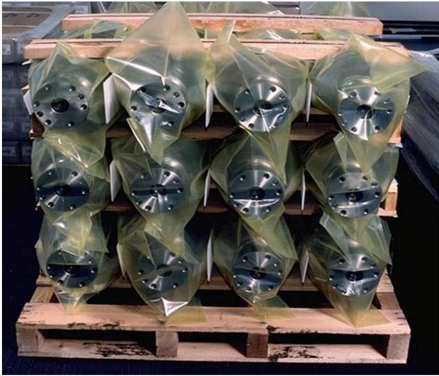
Figure 1 - Clean, oil-free crankshafts, each in a closed VCI bag in layered pallet for ocean shipment to assembly plant.
