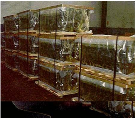
Figure 2 – Engines in sealed VCI bags during long-term storage and subsequent ocean shipment.
