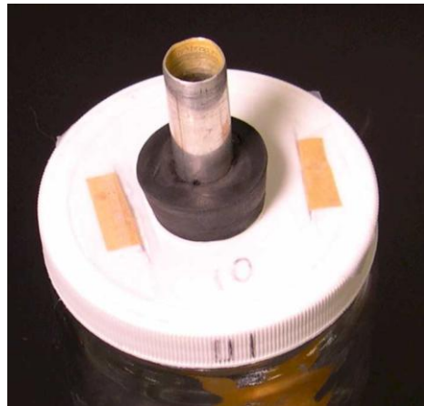
FIGURE 10: VIA-Ferrous test jar lid (external view) showing VCI material sample strips inserted through slots in lid and held in place with low-acid transparent adhesive tape. (11)
