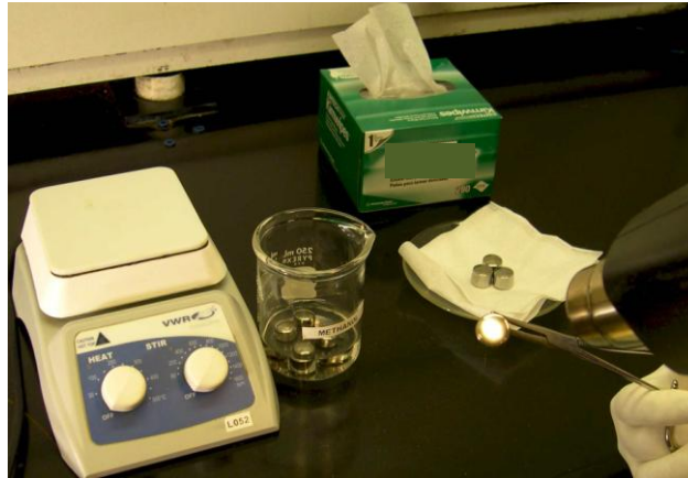
FIGURE 8: Specimen, held with clean forceps in a gloved hand, being dried by a heat gun. Several dried specimens are temporarily held on an absorbent lint-free laboratory wipe. (9)
