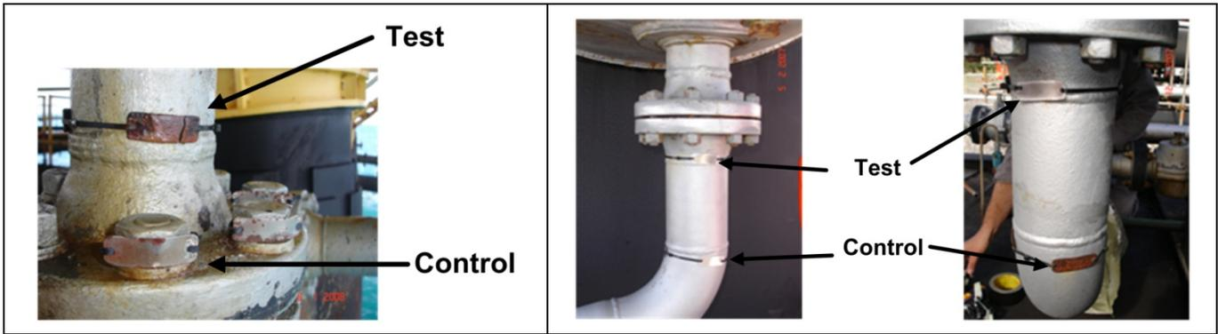
**FIGURE 7 – Brazil Field Trial Specimens: a) Offshore - 11 months;
