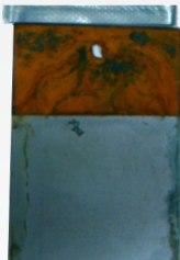
Protected by Zerust VCI Tape for 96 hours
