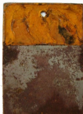
Protected by plain tape for 96 hours
