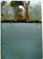
Protected by Zerust VCI Tape for 48 hours
