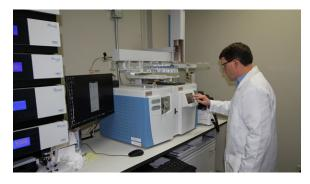
Our GC/LC Mass Spectrometry is just one of the tools we use in our lab for testing a customer's process fluids and the effectiveness of recommended corrosion solutions.
