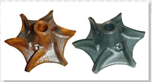
AxxaClean™ ICT®620-RR effectively removes rust on intricate parts by immersion cleaning.
