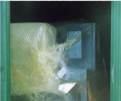
An electrical box protected internally by ZERUST® ICT® Vapor Capsules and externally by ZERUST® ICT®510-C Film.
