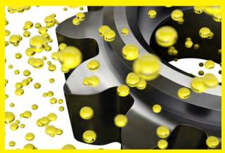
VCI molecules inhibit corrosion by preventing moisture and environmental elements from reacting with the metal surface. Since VCI molecules are transported through the air, they must be trapped around the metal surface using a poly bag or other enclosure. Later, when the enclosure or package is opened, the ZERUST® corrosion inhibiting layer dissipates, leaving clean, dry, and residue-free metals.
