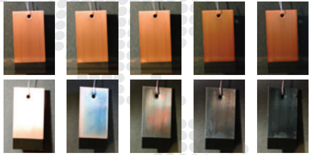
Panel protected by ActivPak in H 2 S sulfur gas environment. (2-18 ppm)
