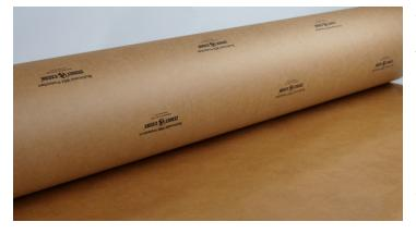
ZERUST<sup>®</sup> ICT<sup>®</sup>432-35P is a kraft packaging paper containing ZERUST<sup>®</sup> Vapor Corrosion Inhibitor Technology (VCI) coated with a 3/4 mil plain polyethylene coating on one side. The plain polyethylene coating provides the kraft paper with increased tear and moisture resistance. Place the plain kraft paper side facing the metal surface to allow the powerful vapor corrosion inhibitors (VCI) to protect ferrous and non-ferrous metal coils.
