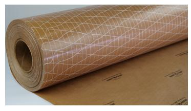
ZERUST<sup>®</sup> ICT<sup>®</sup>430-35SR Scrim Reinforced VCI Paper is a high-quality 35# kraft paper that is saturated on one side with proven ZERUST<sup>®</sup> corrosion inhibitors and laminated with a 3/4 mil polyethylene layer and fiberglass scrim on the backside to provide superior strength. Place the plain kraft paper side facing the metal surface to allow the powerful vapor corrosion inhibitors (VCI) to protect ferrous and non-ferrous metal coils.
