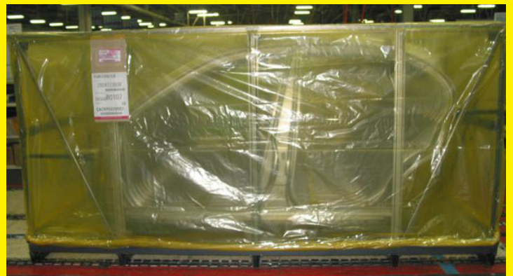
Automotive frame wrapped in ZERUST® ICT®510-C VCI Film for rust-free protection during overseas shipment.
