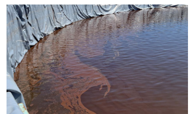
Post-hydrotest discharge showing contaminants, residues, and corrosion byproducts flushed from internal pipe surfaces during testing.
