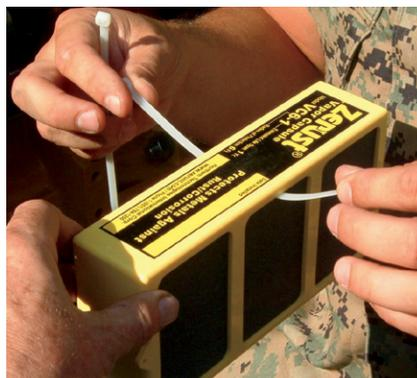
Products with or without adhesive may need to be secured with a cable tie. Particularly when vibration, cold, or surface contaminants may cause the adhesive to be ineffective over time.
