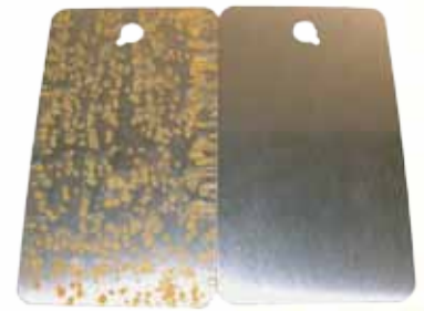
Plate on left was stored in normal poly film; plate on right protected by Zerust VCI Film.
