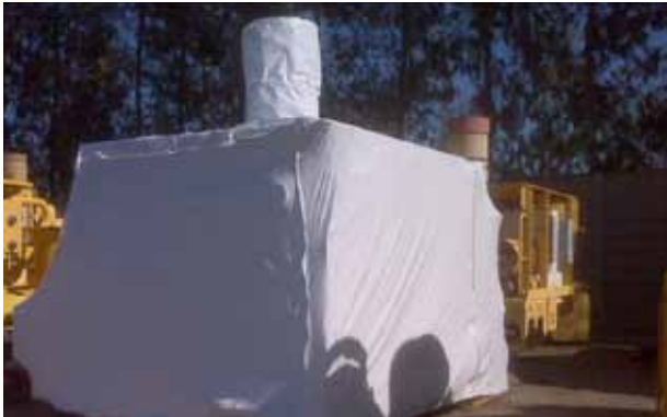
Large machinery shrink-wrapped for long-term outdoor protection.
