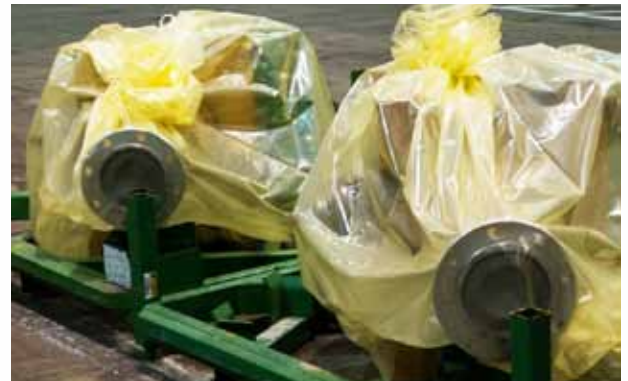
Large assemblies contained in Zerust Gusseted VCI Bags are ready for use, shipment or storage.
