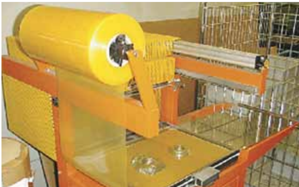
Small parts are securely held to Zerust treated cardboard by Zerust Skin Film.
