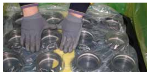
Zerust ICT®520 CSL Cold Seal Film Application
