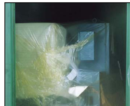
The view inside one container. A large electrical box and related motor and process controls protected externally by Zerust® ICT™510-C Ferrous Film and internally by Zerust® VC6-1 Vapor Capsules.
