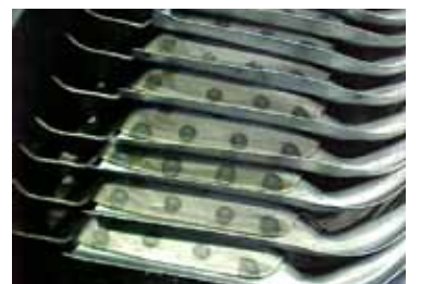
Critical areas, such as welding points, showed no signs of corrosion after being packaged in Zerust® ICT®510-C Film.
