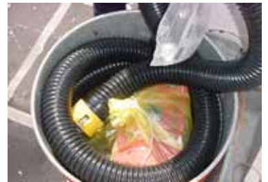
Zerust VCI bags protected bail-out pumps from corrosion until they are needed.
