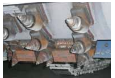
Non-critical area left unprotected by Axxanol Spray-G during shipment. Unprotected area quickly rusted.
