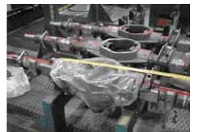
Differential units were quickly and easy wrapped in Zerust cold-seal film.
