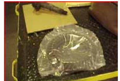
Zerust cold-seal film protecting a large gear for service shipment. Previously parts had been wrapped in VCI film and tape.
