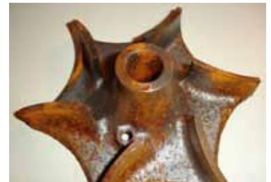
A severely rusted cast iron impeller.
