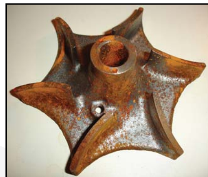
Above: A severely rusted impeller. Below: The same part after treatment with Zerust® ICT™620-RR Rust Remover.
