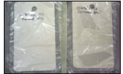
The 1010 steel panels packaged in Zerust® ICT™510-CLHD Film showed absolutely no corrosion after 30 days in the test chamber.
