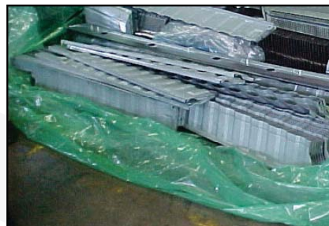
When Zerust® ICT™510-C Film was used, all of the components arrived corrosion free.
