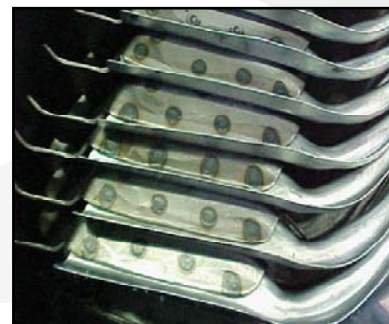
Critical areas, such as welding points, showed no signs of corrosion after being packaged in Zerust® ICT™510-C Film.
