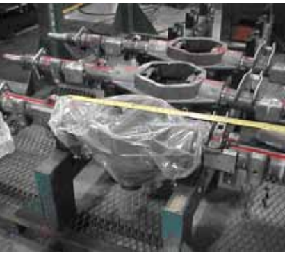
Zerust® ICT®520-CSL Film protecting a differential unit during service shipment.
