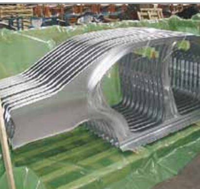
Automotive parts protected with Zerust® ICT®510-C Multimetal Film.
