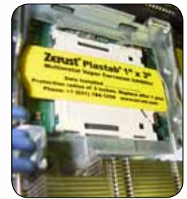
1" x 3" Plastab in an electronic's enclosure
