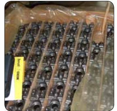
Corrosion-free shipment protected by Zerust
