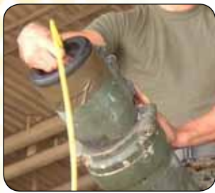
Tube Strip being inserted into a barrel.
