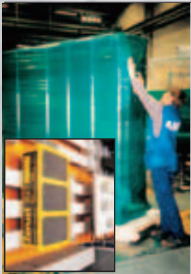
An electrical control cabinet protected inside by ZERUST® Vapor Capsules and protected outside with combination Zerust® Multimetal/Anti-Static film.
