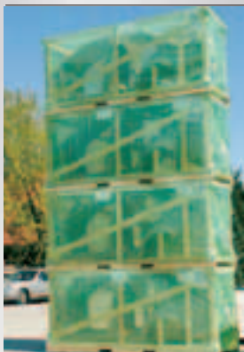
Automotive CKD (Complete Knock Down) components being protected with ZERUST® Multimetal film for intercontinental transit.
