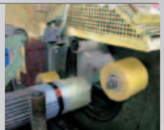
Steel bars being automatically wrapped in ZERUST® Ferrous stretch film.
