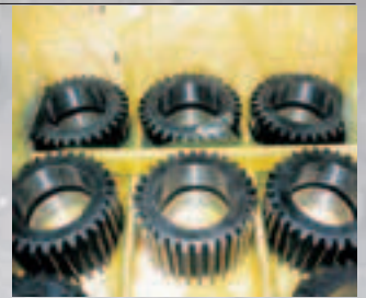
Gears packed in a ZERUST® Ferrous crate liner that covers the interior dividers in order to prevent contact with corrosion-causing wood.
